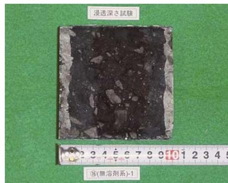
図-3 浸透深さの測定例 (No.5)
